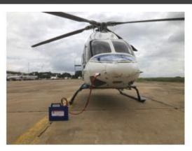
An Ultra-Light Weight, Portable, Smart GPU
