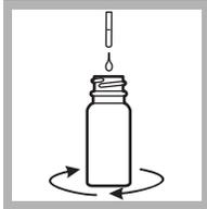
5. Add Sodium Thiosulfate Standard Solution by drops. Count the drops until the color becomes colorless. Swirl to mix after each drop.
